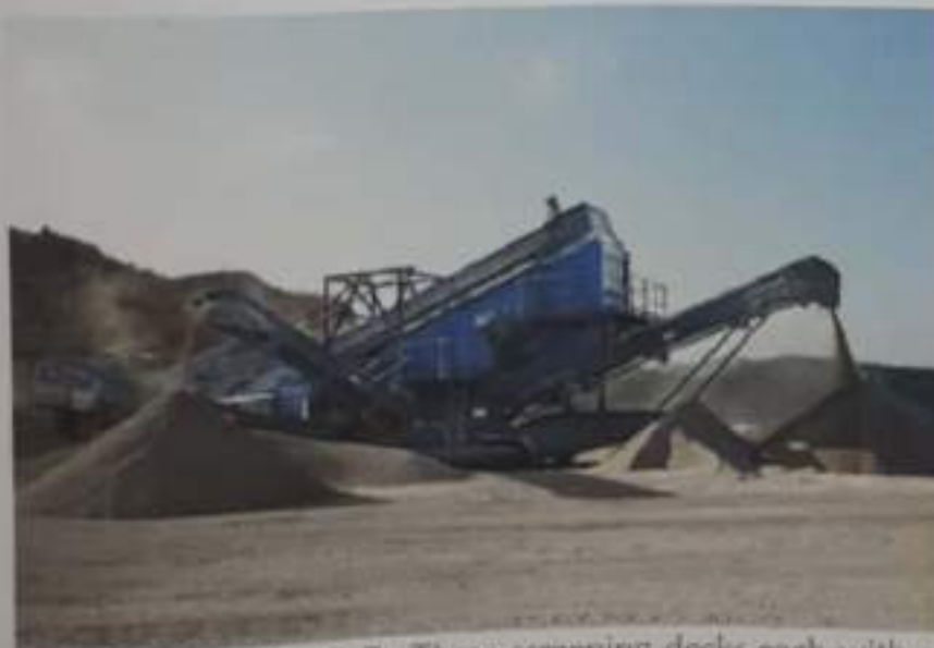
MOBISCREEN M5 20 D: Three screening decks each with a screening area of 12.3 m 2 ensure maximum efficiency, also for smaller grain sizes.
