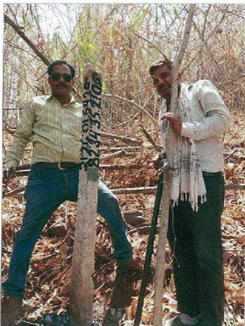
Pillaring after DGPS Survey by Rover
